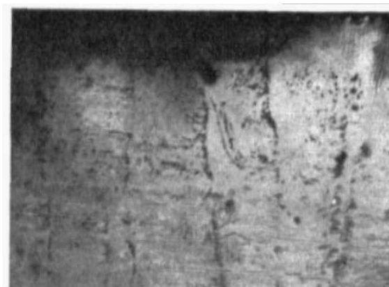
(e) Complicated closure pattern on side of crystal, i.e. (112) plane. Field parallel to [110] direction→
